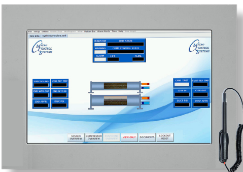
EVAPORATOR CONDENSER OVERVIEW SCREEN
